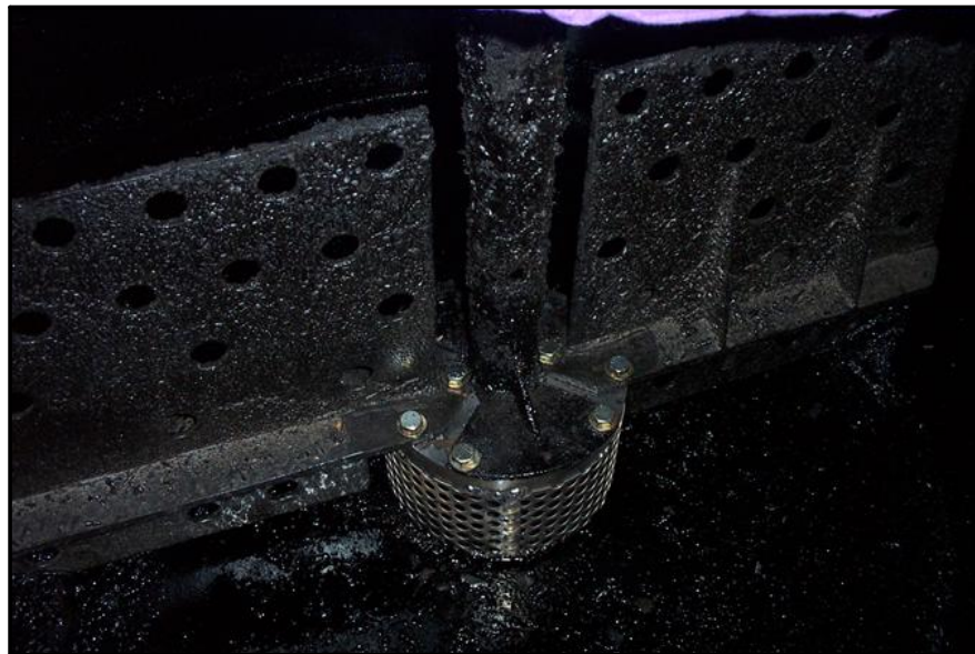
Fig. 6-10 Agitator Shaft and Paddles Mounting
